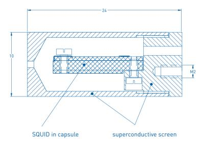
The **Model CCblue** is designed for a simple customerspecific setup of niobium wire wound magnetometers and gradiometers as well as for preamplifiers of current or voltage signals with small amplitudes (e.g. signals of transition edge sensors TES).
